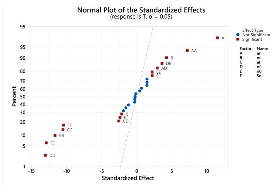
Fig 3. The normal plot of the standardized effects of input factors on wheel life time
