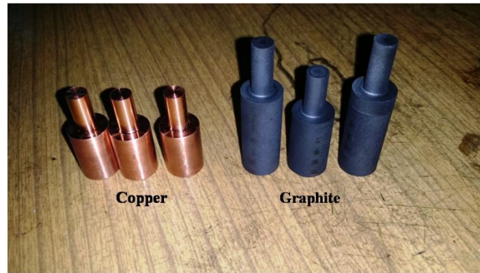
Fig. 1. Copper and graphite electrodes before EDM.
