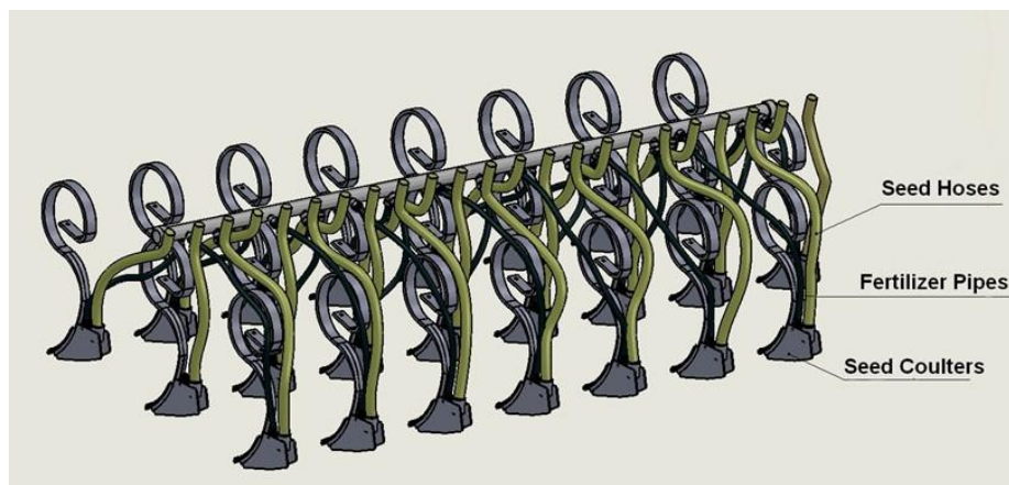
Figure 2. The liquid fertilizer system of the mulch direct grain planter
