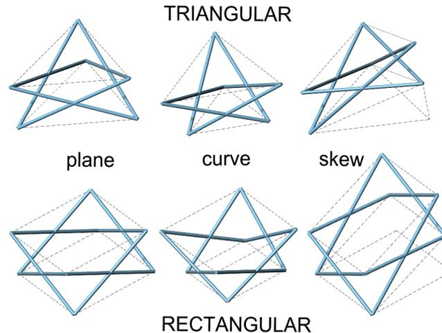
Figure 1. SLE modulus used for expandable structures.
