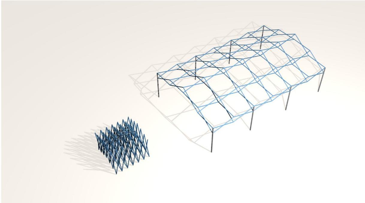
Figure 11. Gable roof folded and deployed
