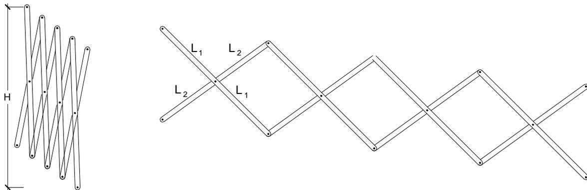
*Figure 5.- Scheme of folding of an oblique module.*
