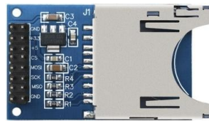
Fig. 6. SD card module used to record measurement results
