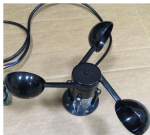
Fig. 5. The sensor used for wind measurement (Anemometer)
